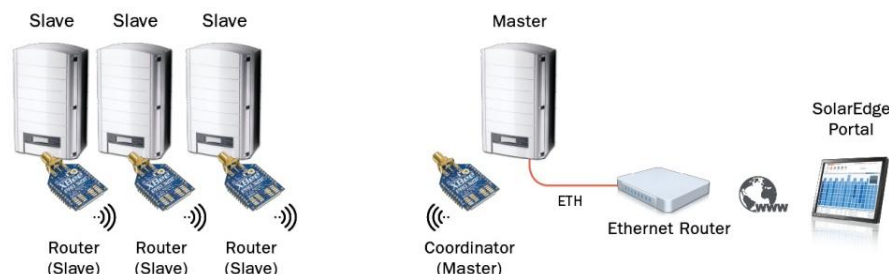
Figure 3: Multiple Devices, ZigBee Bus, Ethernet Server Connection
