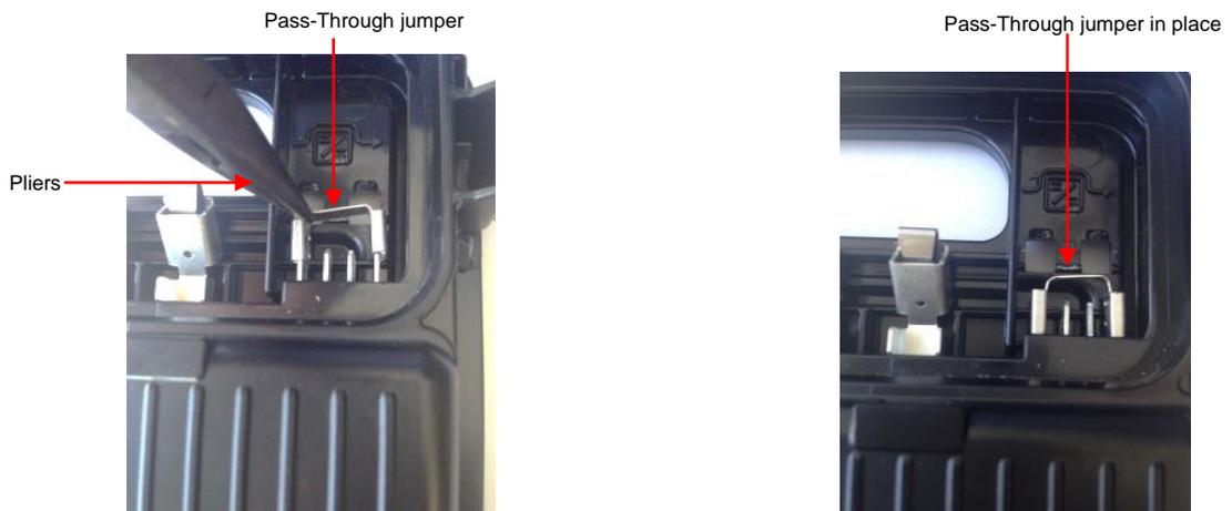
**Figure 6: Inserting the Pass-Through mode jumper**
