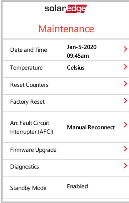
2. Tap **Arc Fault Circuit Interrupter (AFCI)**. The AFCI screen is displayed.
