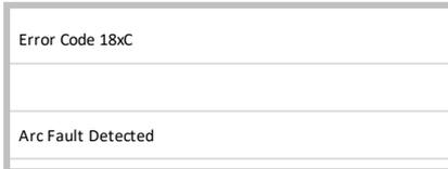
3. Perform manual restart to resume system operation: Turn the inverter ON/OFF switch to OFF and then to ON. The inverter performs an arc detection self-test and starts normal operation. If the test fails, contact SolarEdge support.
