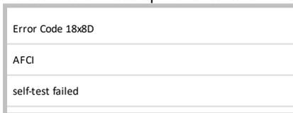
The inverter continuously repeats the arc detection self-test until it is successful.
