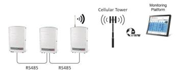
Figure 3: GSM Plug-in high bandwidth mode connection diagram
