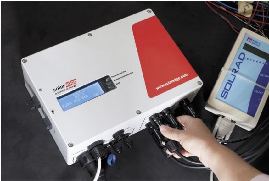
This interface box can be looped in between the supply cables for the strings and the inverter, allowing the system's monitoring functions to work with inverters that are not made by SolarEdge. If anything, this configuration had a positive effect during the lab's tests.
