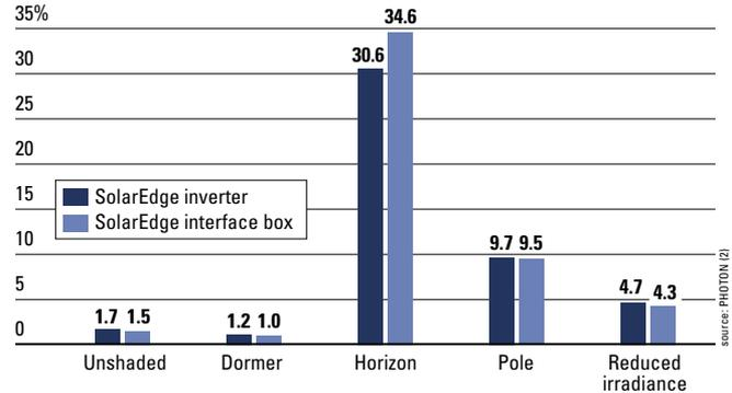
When optimizing a long string, the differences in the results produced by varying shade conditions stand out. The gains are particularly large when there is horizon shading.
