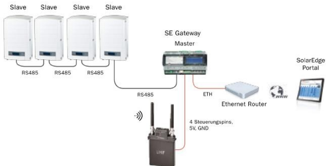
Figure 3 – Scheme of an installation
