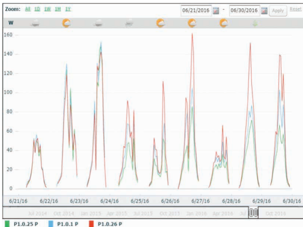
The graph for Site 1 shows failing panels P1.0.25 P , P1.0.1 P compared to reference panel P1.0.26 P .
